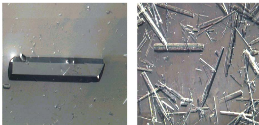
Fig. 2. Microscopic images of crystals of form B obtained from acetone as a representative.
